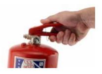
Hold the bottle firmly with one hand and grasp the handles with your other hand. With the bottle pointed in a safe direction, squeeze the handles together to open the valve. You can start off by opening the valve just far enough to bleed off pressure and then open farther as the pressure is released. Close the valve by pulling the handles apart. Your bottle is now ready to ship.
